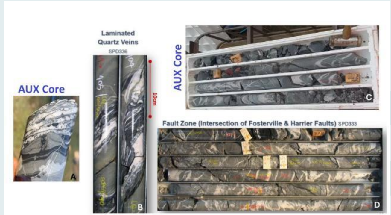
Similarities between Golden Cross (AUX) core and Fosterville drill core. A) Laminated Quartz Vein marker horizon as seen in drilling at Shepherd's Hill. B) Laminated Quartz Veins from Fosterville. C) Fault zone with quartz veining as seen at Shepherd's Hill. D) Fault zone with quartz veining as seen at Fosterville. (Fosterville images taken from Kirkland Lake Gold presentation dated September 2019)
